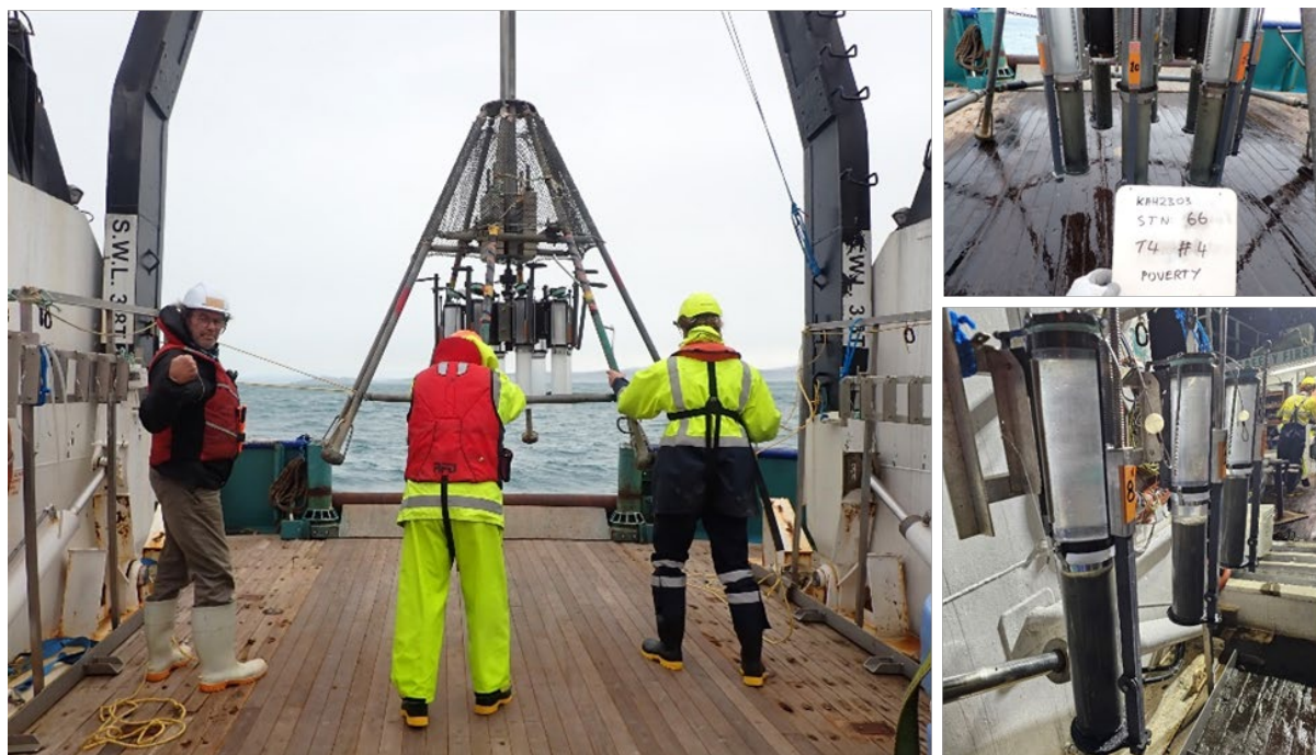
Figure 8: Multicorer deployed from RV Kaharoa to recover sediment cores during the post-Cyclone Gabrielle June survey (left). It can collect up to eight 70 cm long cores simultaneously (right top). Shuttles capturing the core samples are placed in racks for further processing (right bottom).
